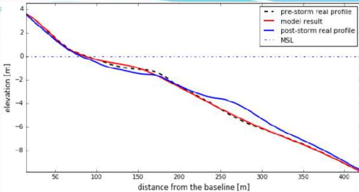
Figure: The difference about cross-shore profile changes between model result and surveyed data of P4.
