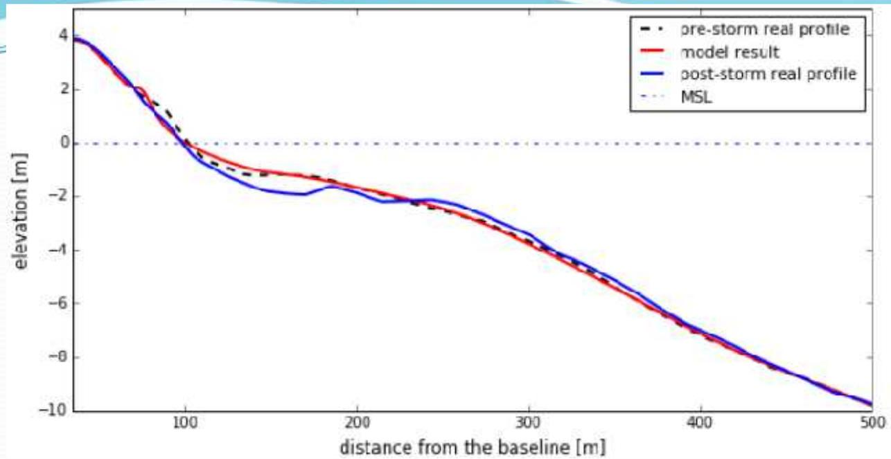
Figure: The difference about cross-shore profile changes between model result and surveyed data of P2.
