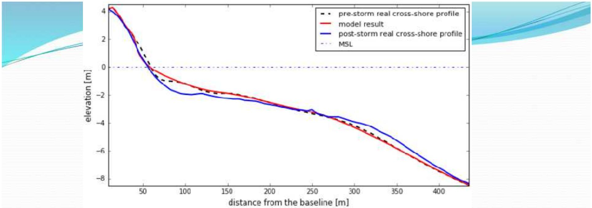
Figure: The difference about cross-shore profile changes between model result and surveyed data of P1.
