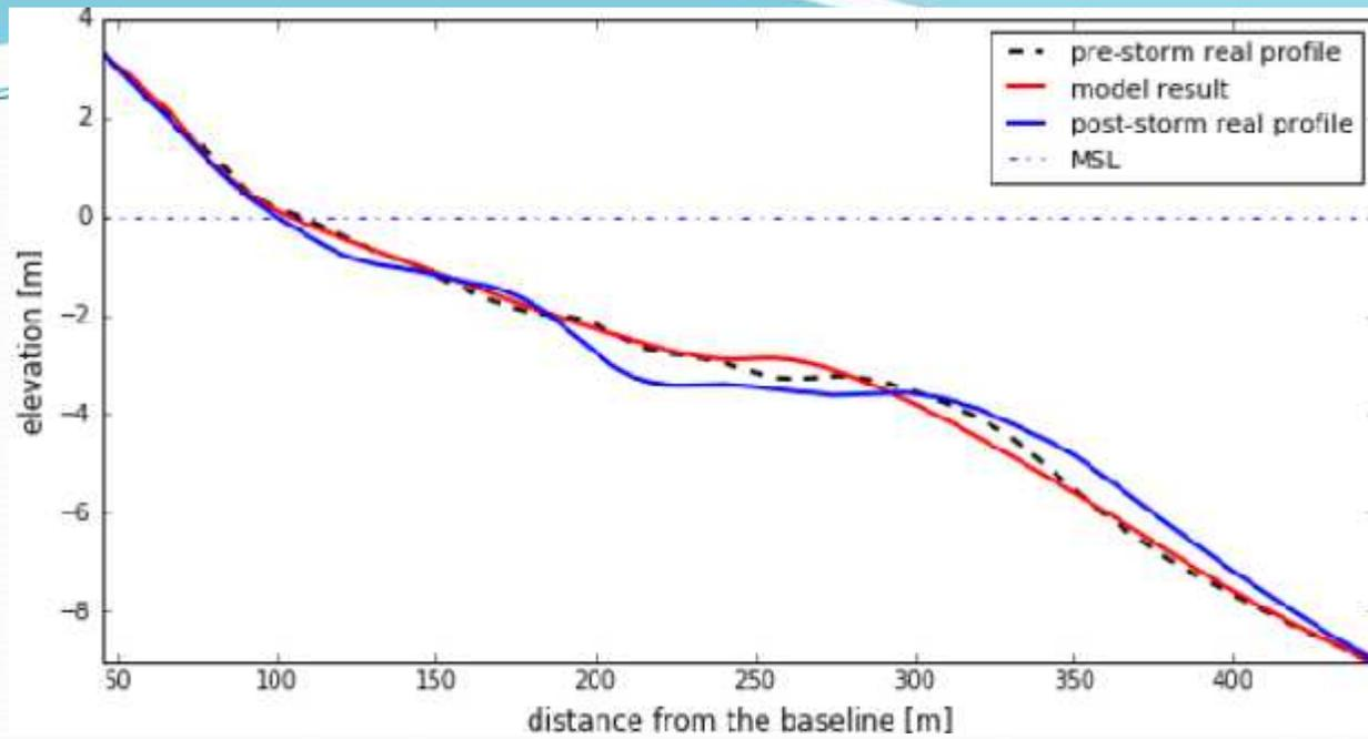
Figure: The difference about cross-shore profile changes between model result and surveyed data of P3.
