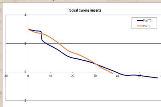
The COPE beach profiles form the basis of any future assessment of the impacts of extreme events such as tropical cyclones. Any erosion of the beach profile is evident from pre and post cyclone surveys.
