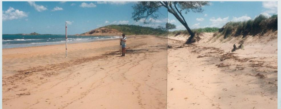
Photos taken with an SLR camera were joined together to give a whole of beach image, note the pole which was used as a reference point for beach profiles, Berm width and wind/wave measurements.
